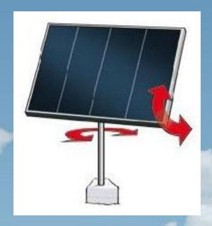
The sun's intensity falls off as the angle between the sun and the face of the panel changes. Convenience and cost generally outweighs the advantage of a tracker!!!!
